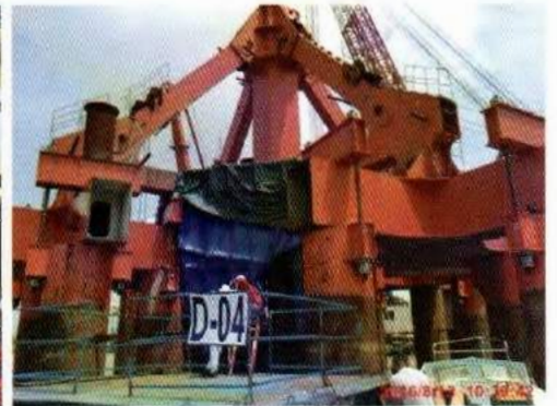
Static load test of TD4A stage-1
